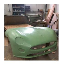
The GRP mouldings are supplied with captive fittings in position. The two bonnet components are test fitted to our Z3 rig and prebonded. The finish is plain gel coat, mould line flash is removed but you need to trim to fit and do final fairing before spraying.
